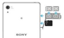
• Make sure you place the nano SIM card (or cards) in the nano SIM card holder before inserting the nano SIM card (or cards) into the device. Also, don't confuse the nano SIM card slot with the memory card slot.
