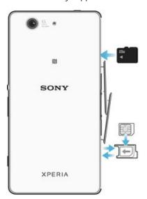
! Make sure you insert the nano SIM card into the nano SIM card holder before inserting it into the device. Also, don't confuse the nano SIM card slot with the memory card slot.
