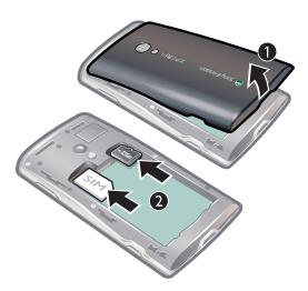
Remove the battery cover, then insert the SIM card and the memory card in the relevant slots.
