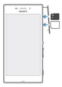
Don't confuse the nano SIM card slot with the memory card slot. Inserting a card in the wrong slot could damage both the card and your device.
