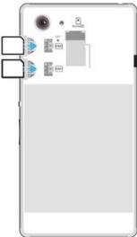
Remove the back cover, then insert the SIM cards into the corresponding slots with the gold-colored contacts facing down.
