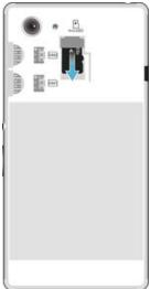
Turn off the device, or unmount the memory card from Settings > Storage > Unmount SD card.
