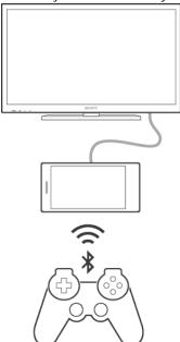
To set up a connection between a DUALSHOCK™3 wireless controller and your device, a USB On-The-Go adapter is required.
