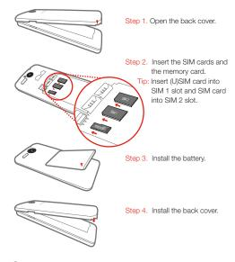
DO NOT insert or remove the SIM cards while your phone is turned on. Doing so can permanently damage your SIM card or your phone.
