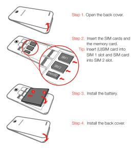
DO NOT insert or remove the SIM cards while your phone is turned on. Doing so can permanently damage your SIM card or your phone. Charge the battery as shown.
