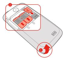
Step 1. Hook your fingertip under the back cover and then pry to open the back cover.
