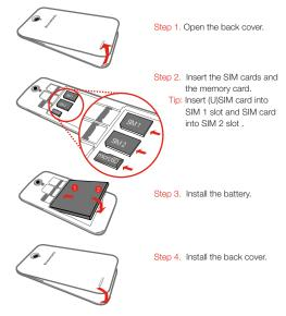
DO NOT insert or remove the SIM cards while your phone is turned on. Doing so may permanently damage your SIM card or your phone.
