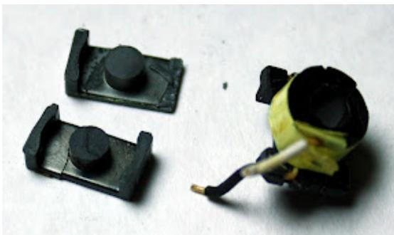
Underneath the next two layers of tape is a 17-turn winding of thin varnished wire, which I think is another shield winding to return stray interference to ground.
