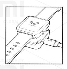
The device is activated by charging, or by pressing the button on the right side of the clock.
