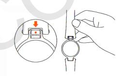
2. Tracker installation into cambered strap
